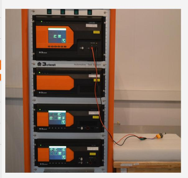
While the electric generator charging to battery, the generator may produce a high energy pulse if battery is disconnected accidently which may cause the damage of automotive devices.
